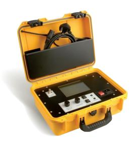
The 406-16 is a self-contained receiver decoder designed to interface with a pair of antennas to provide left/right steering information together with additional bearing, steer and distance information being made available to the rescue craft.
