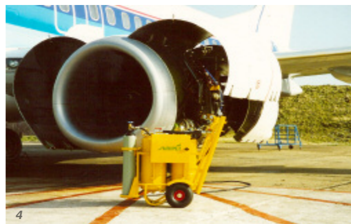
4 Juniper's first lightweight compressor washing rig for commercial engines (JMP/CFM56/D/1535), in use at ATC Lasham Limited, Hampshire on an Air UK Leisure Boeing 737-400 (CFM56-3 engine).
